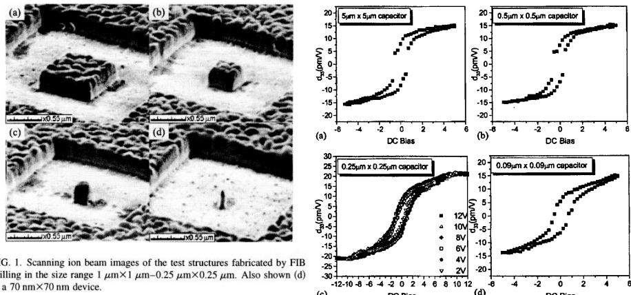
FIG. 1. Scanning ion beam images of the test structures fabricated by FIB milling in the size range  $1 \mu\text{m} \times 1 \mu\text{m}$ – $0.25 \mu\text{m} \times 0.25 \mu\text{m}$ . Also shown (d) is a  $70 \text{ nm} \times 70 \text{ nm}$  device.
