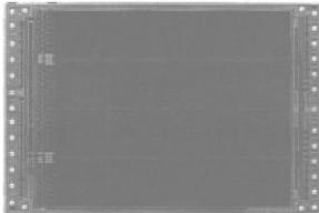
A 256kb FRAM, which consists of four 64Kb arrays. Peripheral circuits locate at the left and right sides of the chip.
