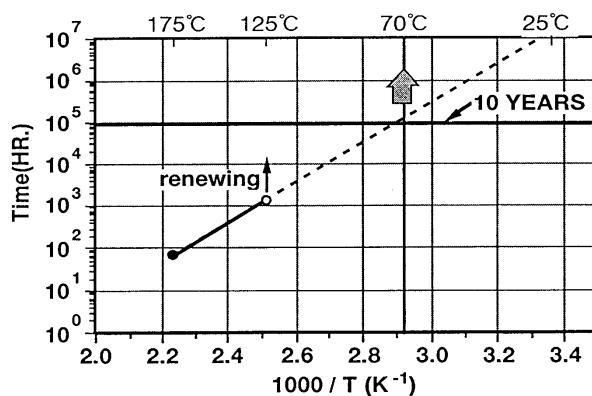
Failure time vs temperature measured on a 256kb 1T/1C FRAM
