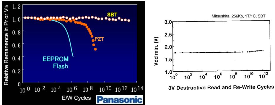
Now the switch endurance of FRAM cells with PZT can reach  $10^{15}$  cycles.
