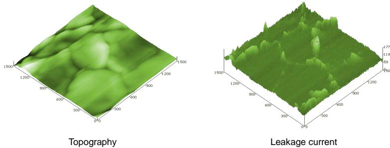
Leakage current along grain boundaries
