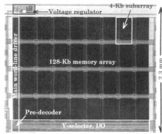
Technology 0.35µm 3-metal CMOS, CMVPP process
