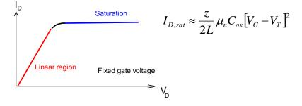
No dependence on  $V_{\rm D}$  so no conductance (current is fixed) but still a transconductance
