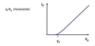
On a linear scale  $I_D$  simply increases with increasing  $V_g$  above  $V_{\ensuremath{\mathcal{T}}\xspace},$  as expected from the previous analysis.
