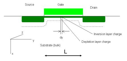
Inversion layer charge  $Q_n$ . Depletion layer charge  $Q_B$ . Channel length L. Channel width z.
