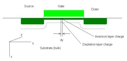
Current flow is continuous from source to drain but voltage drop depends on surface potential.
