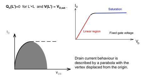
Resistance of inversion layer reduces only slightly, so that  $dl_D/dV_D=1/r_d$  is non-zero (increase slope of dashed line).
