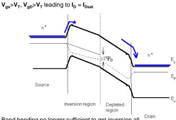
Band bending no longer sufficient to get inversion all <sup>Drain</sup> along channel near to surface.
