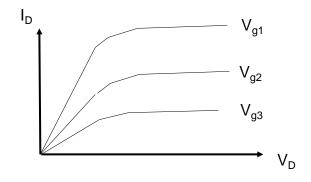
Current essentially independent of  $V_{\text{D}}$  in saturation but still depends on gate voltage.
