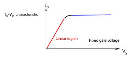
Slope of linear region depends on excess gate drive
