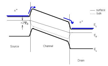
$V_{q}>0$ ,  $V_{p}>0$  (but small), leading to resistive drop in channel.
