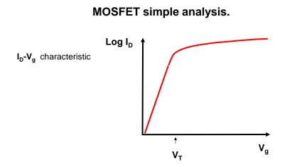
On a log scale  $I_D$  is seen to deviate from this behaviour at low gate voltages, particularly below  $V_7$ , where simple analysis predicts  $I_D$ =zero.
