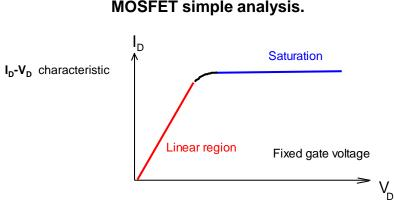
Linear region occurs at low drain voltages where the channel is continuous between the source and the drain.
